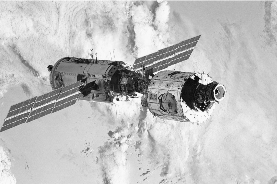
Figure No. A-15. View of the ISS with the Zarya module (left) connected to the Unity module (right), December 1998.
